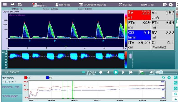
Monitoring screen with M-mode display. The large blue signal in the M-mode screen is the proof of the proper positioning of the probe.
